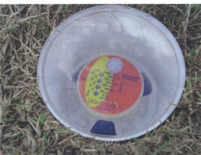
The DLI100 measures light quantity over a 24-hour period and returns a DLI (Daily Light Integral) value.
